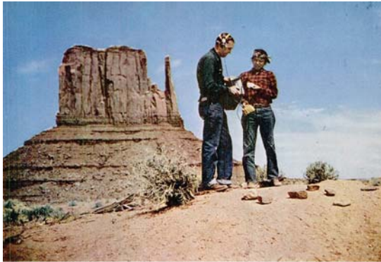
Trader Goulding shows Navajo prospector how a Geiger counter reveals radioactivity in piece of uranium ore PHOTO BY THOMAS E. STIMSON, JR.
